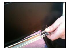
...once the tab reaches the side of the drawer lift the front of the drawer upwards and runner should come away. *Repeat this on both sides*
