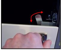
The lock in the bottom drawer turns a metal cam upwards (Drawer above has been removed for illustration purposes)
