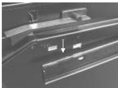
2. Push the front of the slide down to release the front 'tag lancing'.
