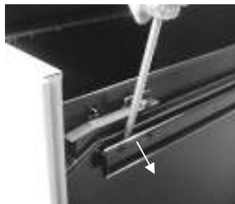
1. Using a slot headed screwdriver lever the slide retaining pip away from the slot in the drawer body.
