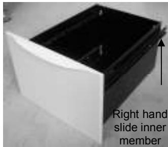
To fit: Support the weight of the drawer while you re-align both slide inner members into the slide centre member bearing cages, and push the drawer shut. (This can be awkward until practised)
