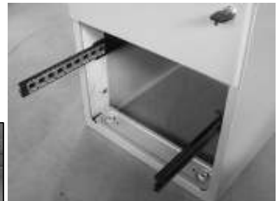
Push the right hand release clip downwards, while pushing the left hand side release clip upwards, and pull the drawer away from the cabinet. (Supporting the weight of the drawer)
