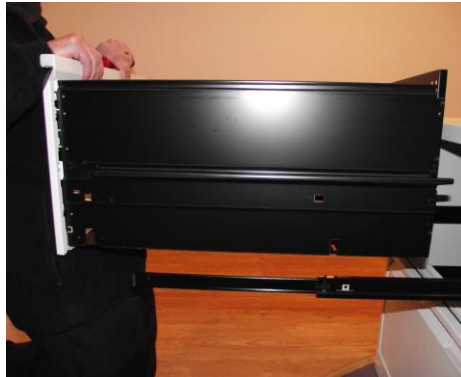
Gently lower the drawer in between the runners.
