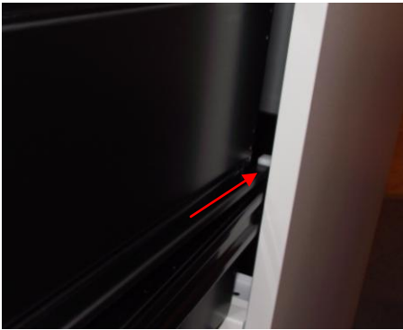
To do this tilt the drawer backwards as far as possible and place the ridge beneath the pin. You can use a screwdriver to lift the locking pin slightly if you are having trouble.
