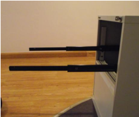
Extend both drawer runners fully.
