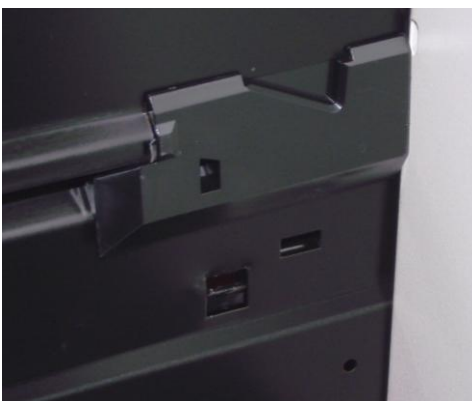
You can then reinsert the front lancements into each side of the drawer....
