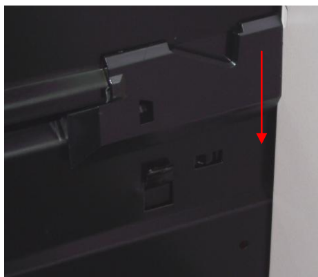
... and push downwards to lock into place. The retaining pip should then rest into its cutout.
